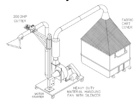
The MITS-CCF-MX is a Move-it-Trim-System Cutter-Cart-Fan for Matrix Removal.
