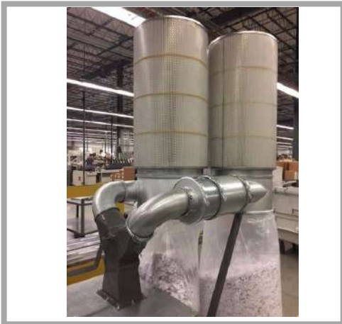
The AirFlex with independent pedestal mounted controls + standard dust containment
