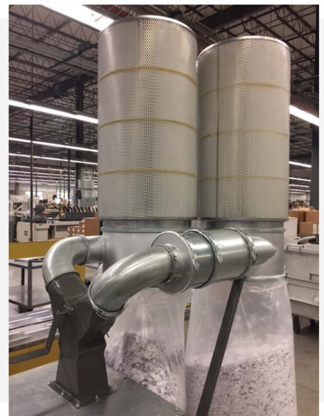
The AirFlex with independent pedestal mounted controls + standard dust containment
